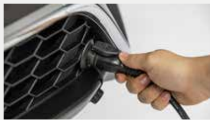
Inline Block Heater + WarmUp system 1) Fully charged battery, warmer engine and warmer compartment Operated by DEFA app on your smartphone or with an In-car controller
